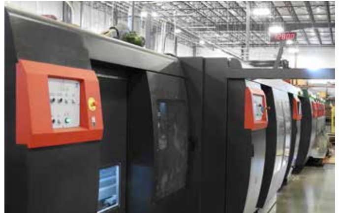
American Box's 'Darth Vader,' EDF Europe's 4-color flexo folder gluer from Haire Group, can produce 24,000 pieces per hour.
